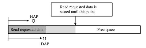
3) When reading of read requested data is completed and transfer of the read requested data to the host system is completed, reading of the disk continues until a certain amount of data is stored.
